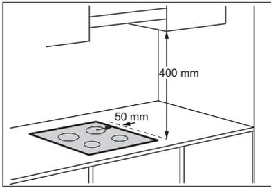
**i** If a furniture unit is installed at a distance of 400 mm above the hob, there must be a minimum safety distance of 50 mm to the left or right from the edge of the hob.
